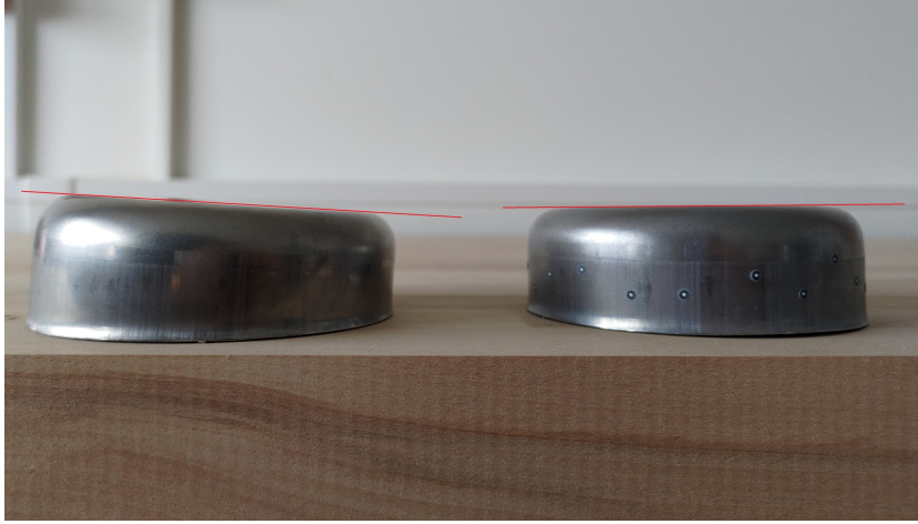
Fig. 9: The eccentricity problem creating tilted bottom of a cup (left) compared to a well formed cup (right)
