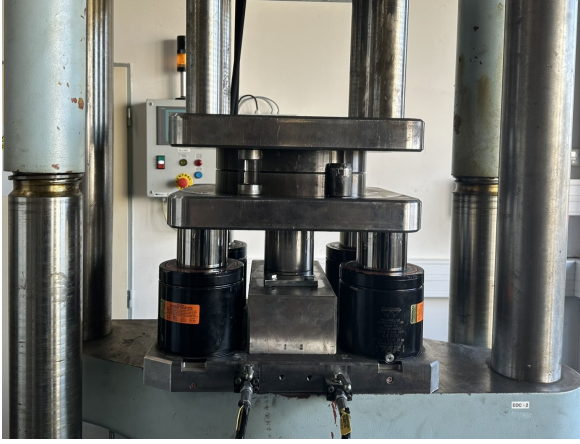
(a) Testing device for deep drawing test
